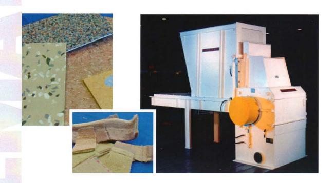
The ORIGINAL PALLMANN Horizontal Knife Mill, type PSRH, called "Biber", with an hydraulic feed system is best suited for the size reduction of most various types of carpet and floor coverings such as edge trims, tiles, sheets or skelletons waste from the production.
